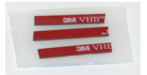
Tape to secure wires.
